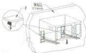
**ENG** Install the other bracket as the same method on the wall. Make sure the two brackets on a straight line at the same level. Put the sticky pad on the beam as shown in the fig. Then set the microwave on the brackets slowly and safely
