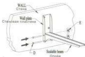
**ENG** Put the beam on bottom of the wall plate, insert the screws through the holes of the wall plate and beam, fix the two nuts to the screws on the other side of the wall plate. Then insert the two plastic cap onto the head of the screw.
